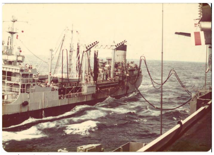
**Supply/Refueling Ship -** *Intrepid* being refueled by an oiler.
